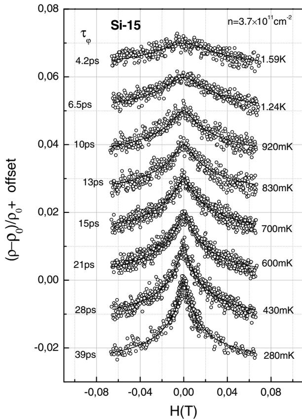
FIG. 1. Change of resistivity versus perpendicular magnetic field for sample Si-15 for eight temperatures at  $n = 3.7 \times 10^{11} \text{ cm}^{-2}$ . The solid lines are fits to weak localization according to Eq. (1).
