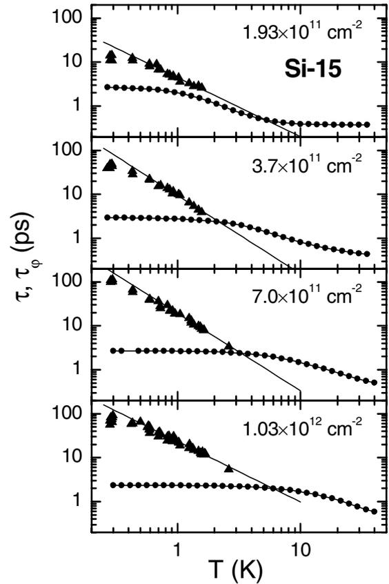
FIG. 2. Experimental temperature dependence of phase coherence time  $\tau_\phi$  (triangles) and momentum relaxation time  $\tau$  (circles connected by lines) for sample Si-15 at  $n = (1.93, 3.7, 7.0, \text{ and } 10.3) \times 10^{11} \text{ cm}^{-2}$ . The thin solid line represents a  $T^{-p}$  least mean square fit to the data points.
