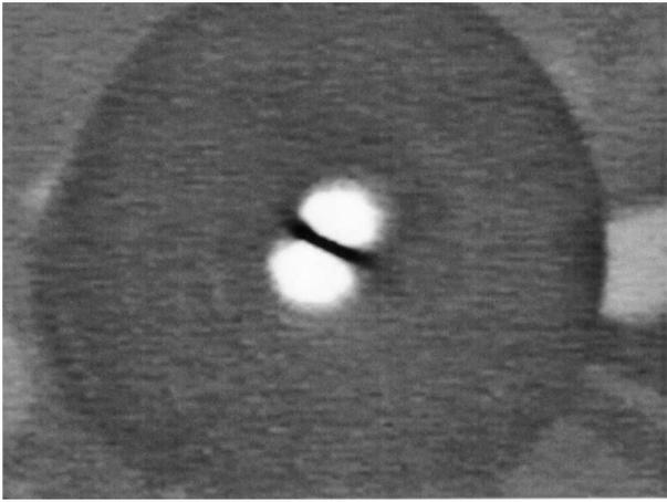
FIG. 4. Infrared impinging on the optical beam dump showing the second harmonic  $TEM_{01}$  mode. The image is tilted due to relative misalignments in the system with perhaps additional contributions from coupling due to misalignment in our optical collimator.
