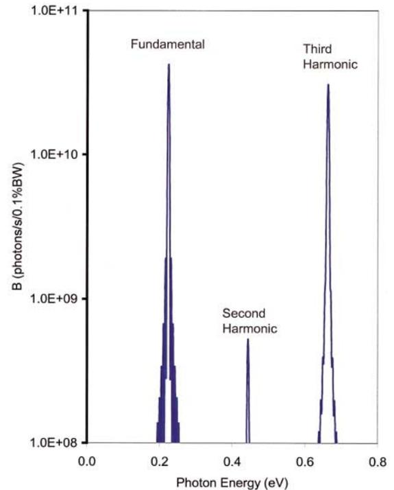
FIG. 1 (color). Calculated spontaneous spectrum of electron beam passing through the JLab wiggler when observing on axis. Calculations performed with SRW [15].
