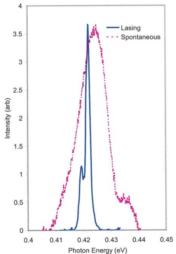
FIG. 3 (color). Second harmonic lasing spectrum displayed with the spontaneous spectrum under the same conditions. The vertical scales are arbitrary. The maximum average lasing power was 3 W. The predicted spontaneous power is on the order of nanowatts but was not measured.
