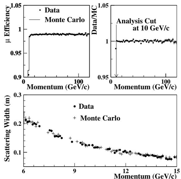
FIG. 1. Muon detection efficiency vs track momentum (top left), data to Monte Carlo ratio of muon efficiency (top right), and multiple scattering width vs track momentum (bottom). Widths are those of Gaussian fits to the difference between extrapolated track position and hit counter position.
