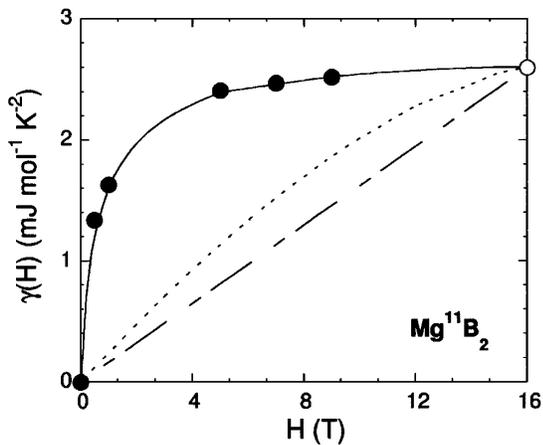
FIG. 2.  $\gamma$  as a function of  $H$ . The solid curve is a guide to the eye and an extrapolation to  $H_{c2}(0)$ . The dashed curve is a “fit” with an  $H_{c2}$  anisotropy of 10.
