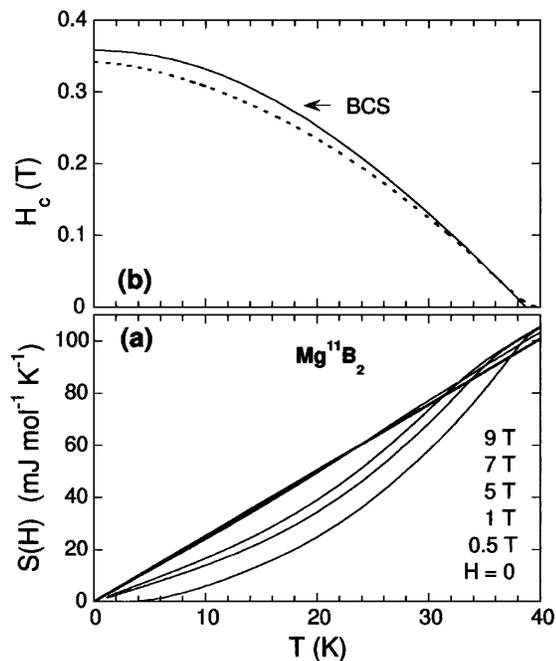
FIG. 3. (a) Entropies as functions of  $T$  for different  $H$ , with  $H$  increasing from the lowest to highest curve. (b) Thermodynamic critical field, compared with a BCS curve for the derived values  $\gamma_n$  and  $T_c$ .
