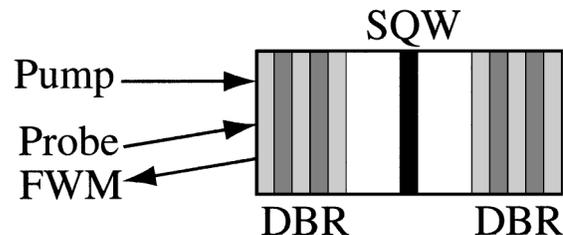
FIG. 3. Schematic of the microcavity four-wave mixing configuration (DBR = distributed Bragg reflector; SQW = single quantum well).
