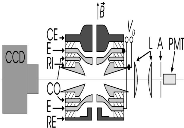
FIG. 1. Schematic of the hyperbolic trap used in the present experiments. CCD is a cryogenically cooled CCD camera, CE is the capture electrode, E are the end cap electrodes, RI is the ring electrode, CO are the compensation electrodes, RE is the release electrode, L are optical lenses, A is an aperture to block stray light, and PMT is a photomultiplier tube.  $V_0$  is the voltage applied between E and RI to create the quadratic electric potential along the magnetic field.
