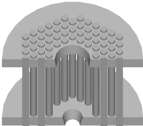
FIG. 1. A section of the computer aided design drawing of the PBG resonator used in the gyrotron experiment. The small aperture on the lower end plate forms the input cutoff section and the bigger hole on the upper end plate is used to extract the radiation from the cavity.
