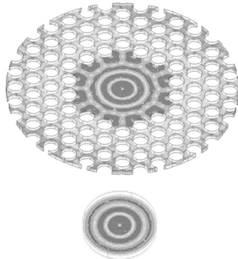
FIG. 2. Comparison of the TE<sub>041</sub>-like eigenmode of the PBG cavity (top) and the TE<sub>041</sub> eigenmode in a conventional cylindrical cavity (bottom). The above simulations showing the magnitude of the electric field were performed using HFSS. The darker regions indicate a higher electric field intensity. The PBG structure is 23 mm in diameter while the cylindrical cavity is 9 mm in diameter.
