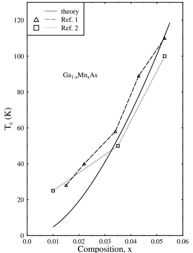
FIG. 1. Mn concentration dependence of ferromagnetic transition temperature in GaAs(Mn). Theoretical dependence (solid line) is obtained from the percolation threshold [Eq. (2)] for  $J_{p-d} = 2.8$  eV,  $\Delta = 0.11$  eV,  $m = 0.53m_0$ .
