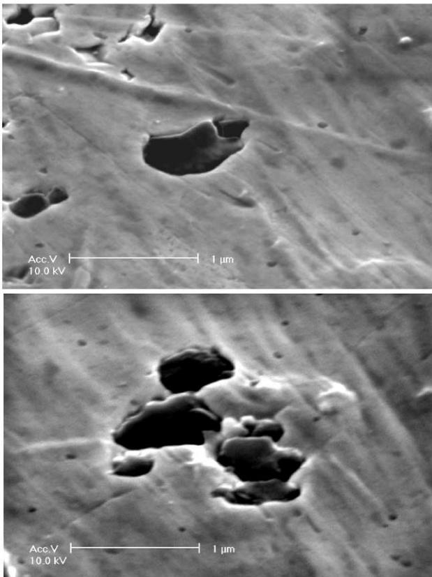
FIG. 1. SEM micrographs of the magnesium diboride grains (dark) embedded in the gold substrate. Typical grain sizes are between 0.5 and 1  $\mu\text{m}$ , thus much larger than the superconducting coherence length.
