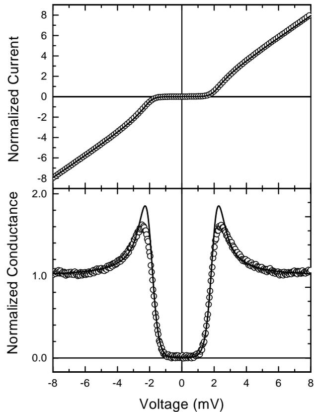
FIG. 2. Experimental (open circles) tunneling  $I$ - $V$  characteristic curve and its differential conductance, normalized to  $R_N = 2.5$   $\text{M}\Omega$ . The solid line corresponds to a BCS normal-superconductor tunnel curve with a gap of  $\Delta = 2.0$  meV and  $T = 2.5$  K.
