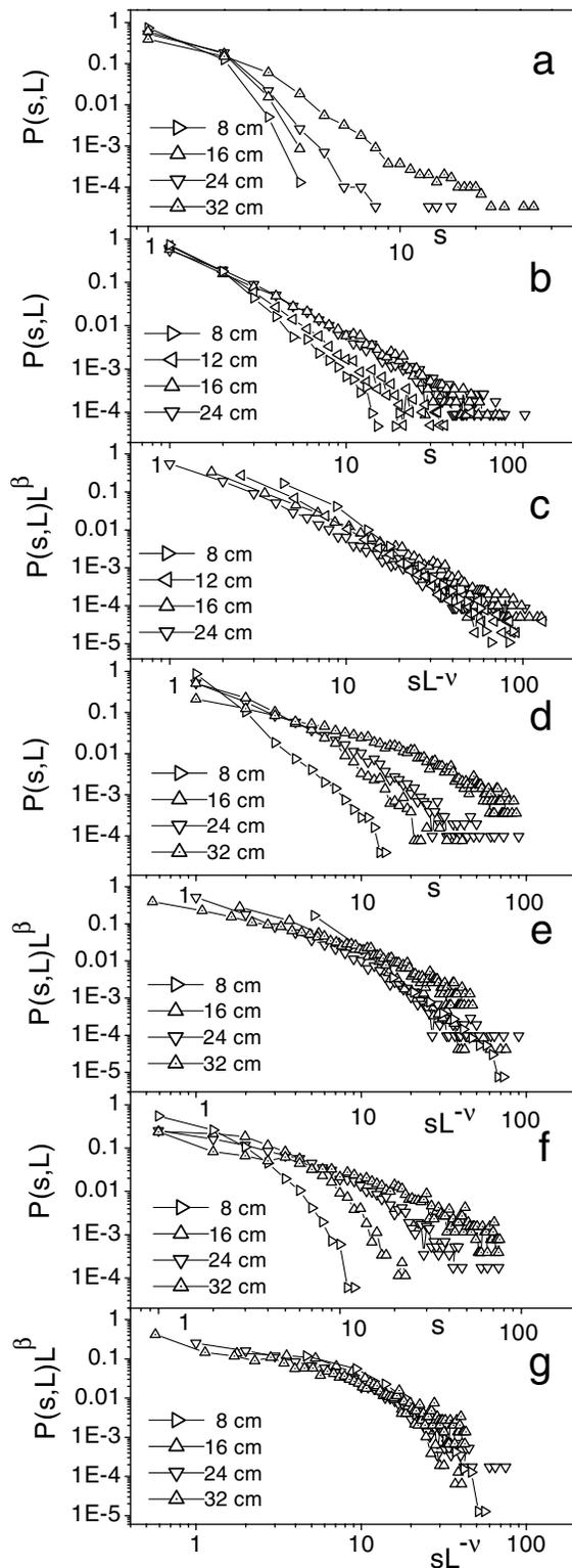
FIG. 2. Avalanche size distributions (normalized to the total number of nonzero avalanches) for (a) Gap3, (b) Gap0, (d) Gap1.6, and (f) Gapan. The scalings based in ansatz  $P(s, L) = L^{-\beta} f(s/L^\nu)$  with  $\beta = \nu = 1.35$  are shown in (c) Gap0, (e) Gap 1.6, and (g) Gapan. It was not possible to obtain any reasonable collapse for Gap3 piles.
