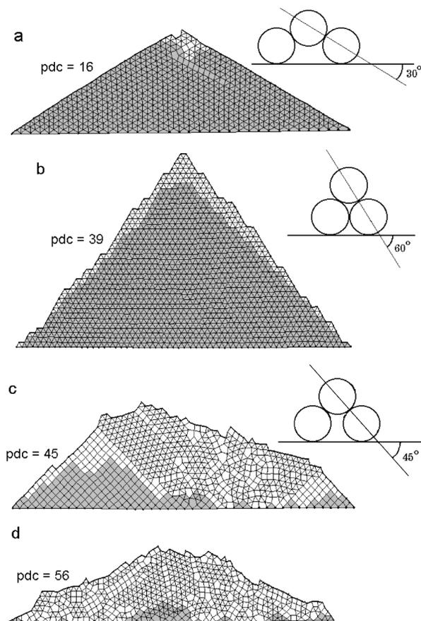
FIG. 1. Schematic representations of typical Gap3 (a), Gap0 (b), Gap1.6 (c), and Gapran (d) piles for  $L = 24$  cm. The heavy dots at the base of each pile represent the centers of beads stuck to an acrylic strip. Triangulations based on the centers of the beads were performed to underline the structural features of the piles. The insets in (a)–(c) display the “ideal” structures of packed spheres. The corresponding “profile disorder coefficients” are also included.
