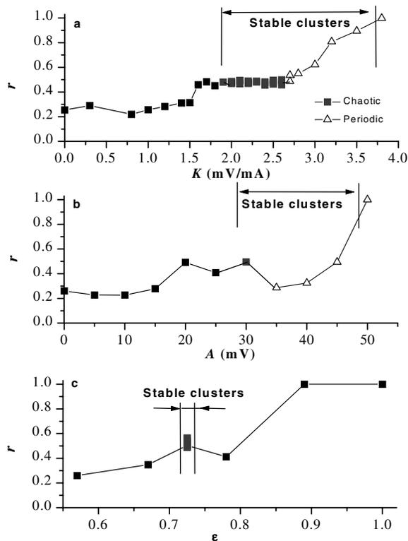
FIG. 4. Order parameter  $r$  based on mean distance as a function of global coupling strength. (a) Feedback. (b) Forcing. (c) Global coupling.
