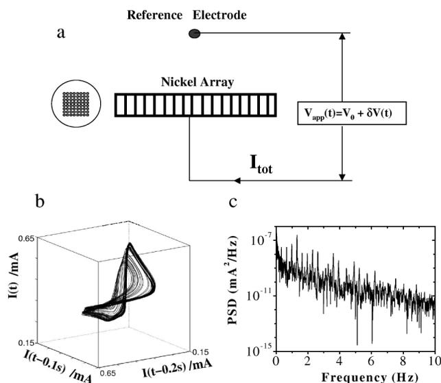
FIG. 1. (a) Schematic of the apparatus. (b) Reconstructed chaotic attractor of the current of one of the uncoupled oscillators. (c) The corresponding power spectrum.
