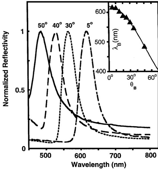
FIG. 3. Normalized reflectivity spectra for various Bragg angles. The inset shows the wavelength of the Bragg band,  $\lambda_B(\theta_B)$ . The solid line is a fit using the relation,  $\lambda_B(\theta_B) = 2d\sqrt{n_{\text{eff}}^2 - \sin^2\theta_B}$ , with  $d = 243$  nm and  $n_{\text{eff}} = 1.3$ .
