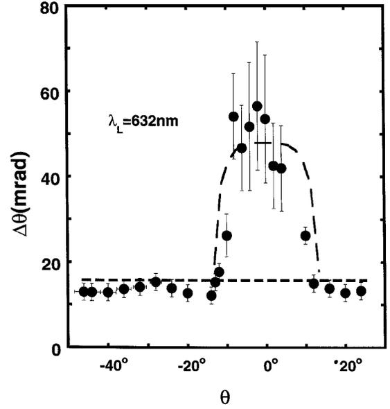
FIG. 4. The effective width,  $\Delta\theta$ , of CBS cones measured at various  $\theta$  around  $\theta = 0$  using  $\lambda_L = 632$  nm, for which  $\theta_B \approx 0$ . The dashed line is calculated using Eq. (4).
