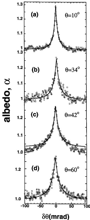
FIG. 1. Coherent backscattering cones in the albedo,  $\alpha$ , at various incident angles,  $\theta$ , measured at  $\lambda_L = 515$  nm: (a)  $\theta = 10^\circ$ ; (b)  $\theta = 34^\circ$ ; (c)  $\theta = 42^\circ$ ; (d)  $\theta = 60^\circ$ . Also shown are fits to the experimental data using Eq. (1).
