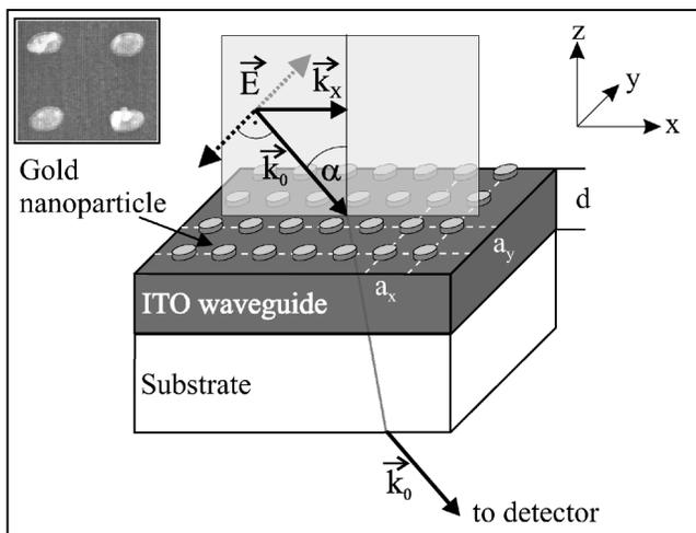
FIG. 1. Sketch of sample geometry. Inset: SEM picture of a gold nanoparticle array on a 140-nm-thick ITO waveguide.
