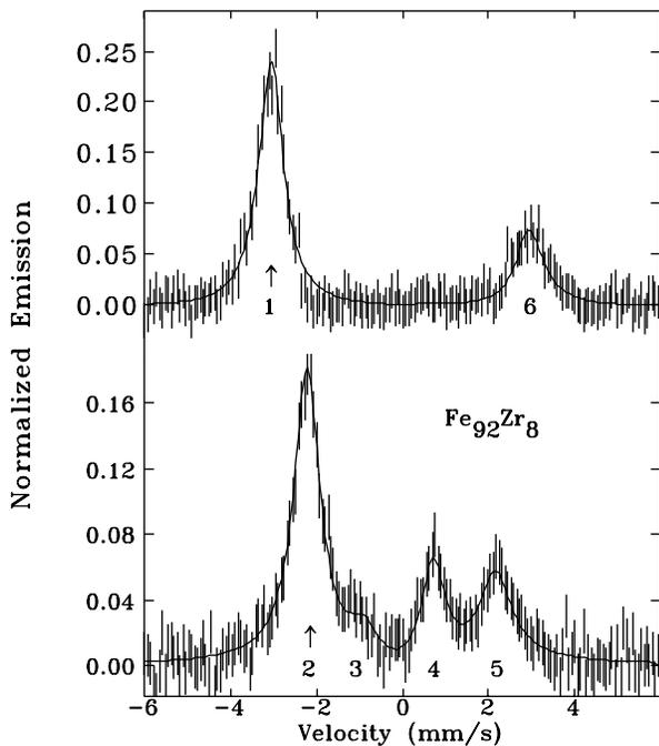
FIG. 3. SEDM spectra at  $T_{xy} = 80$  K when the  $m_e = -\frac{3}{2}$  state is populated (top) and when the  $m_e = -\frac{1}{2}$  state is populated (bottom). Pump energies are indicated by the  $\uparrow$ .
