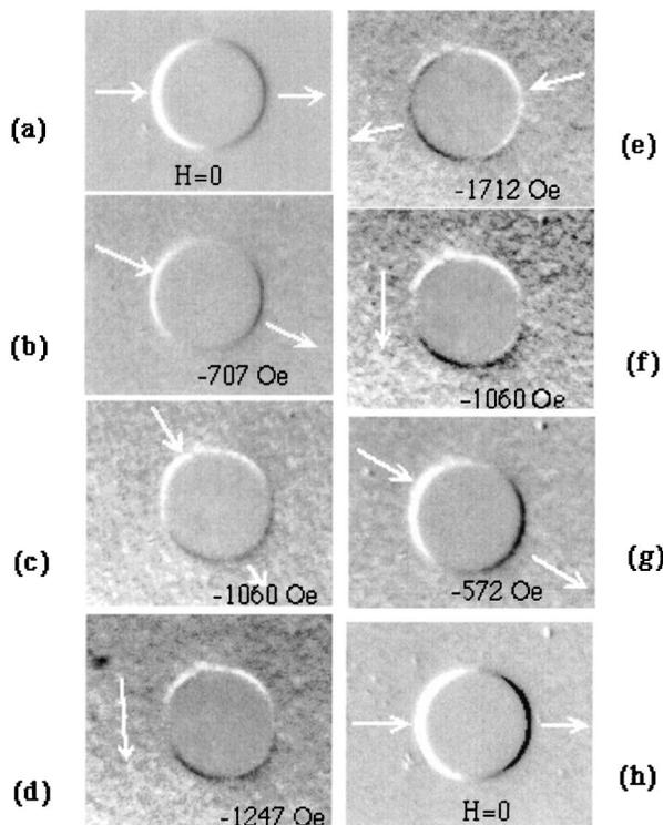
FIG. 1. Magneto-optical patterns around a hole during application of a negative field ( $H$  values shown on the pictures) to the SmCo/Fe structure polarized horizontally by +7 T.
