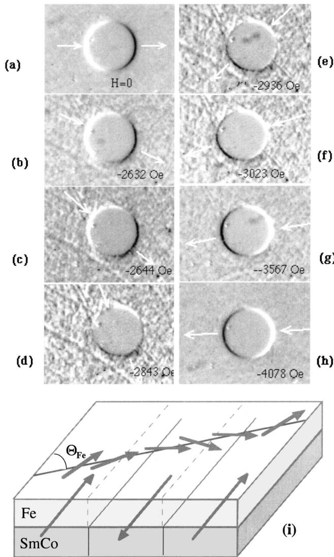
FIG. 3. (a)–(h) Remanent state after application of negative fields shown on the pictures. (i) Schematic of magnetization distributions in Fe and SmCo layers at the partial remagnetization of SmCo. Oscillations of  $\mathbf{M}_{\text{Fe}}$  around the average angle,  $\Theta_{\text{Fe}}$  are shown.
