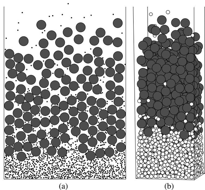
FIG. 1. Brazil nut problem in 2D (a) and 3D (b). Particles with the larger diameter rise to the top. Note that  $T_c(B) < T < T_c(A)$  and percolation overrides the condensation effect.
