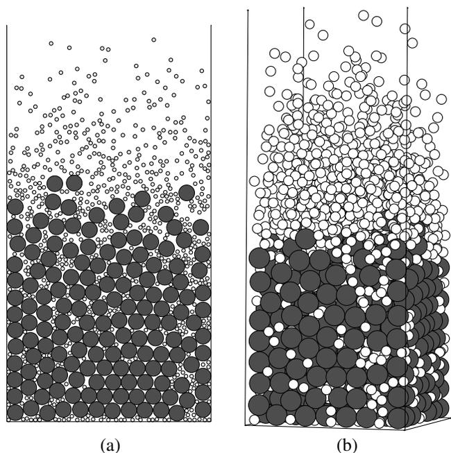
FIG. 3. (a) RBNP along path 1 in 2D. Particles with the larger diameter sink to the bottom. The mass ratio is the same as in Fig. 1a, but the diameter ratio decreased to  $d_A/d_B = 2$ . (b) RBNP along path 2 in 3D. The diameter ratio is the same as in Fig. 1b, but the mass ratio is increased to  $m_A/m_B = 6$ .
