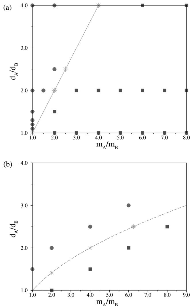
FIG. 4. Phase diagram determined for the segregation of binary mixtures in (a) two dimensions, and (b) three dimensions. In 2D, the straight line is  $y = x$ , while in 3D, the curve is  $y = \sqrt{x}$ . The circles are data points for BNP, the squares for RBNP, and the stars are data points for the mixed state.
