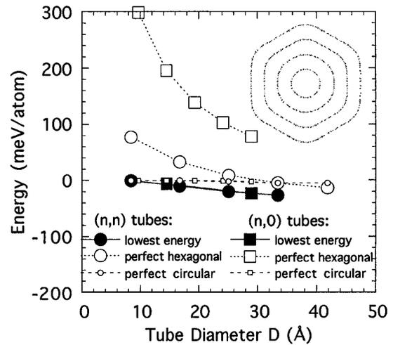
FIG. 2. Energy of the lattice with respect to isolated tubes. Lowest energy tubes are nearly circular for low  $D$  and almost hexagonal for large  $D$ . The inset shows, superimposed, the structures of the lowest energy  $(n, n)$  tubes.
