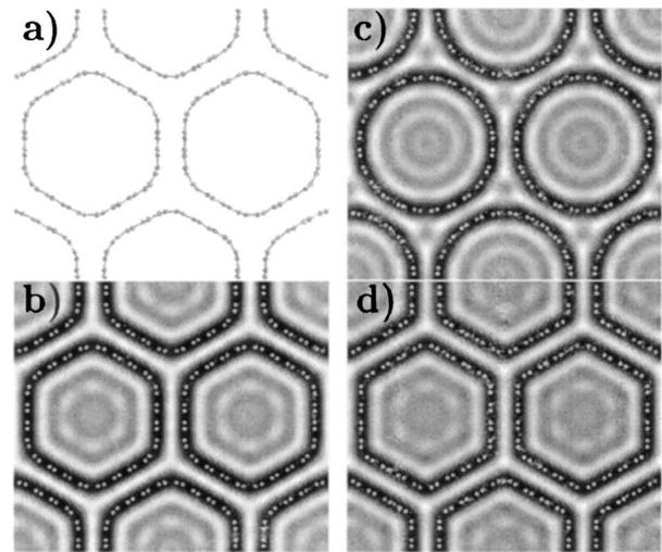
FIG. 3. Simulated TEM images of the plane perpendicular to the tube axes for a lattice of (12,12) tubes with (b) rounded-hexagonal (c) circular and (d) hexagonal cross sections. (a) The atomic positions for configuration (b).
