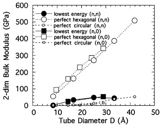
FIG. 5. Two-dimensional bulk modulus in the plane perpendicular to the tube axis of the perfect hexagonal, perfect circular, and lowest energy lattices as a function of tube diameter.
