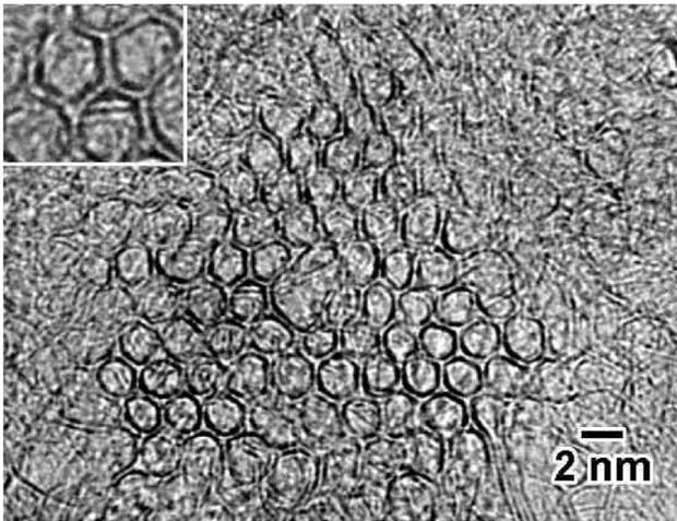
FIG. 1. HRTEM image of a lattice of polygonized tubes produced by  $\text{CO}_2$  laser ablation.
