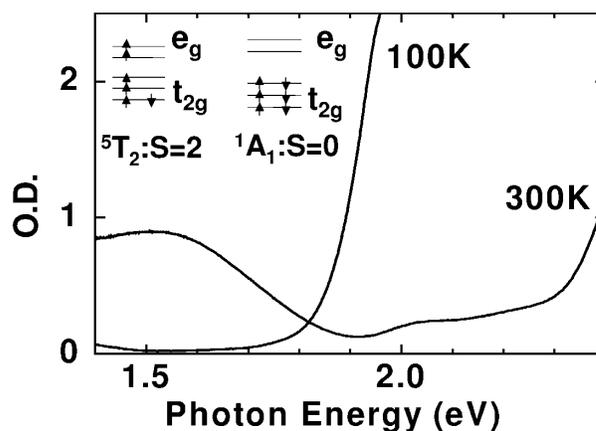
FIG. 1. Absorption spectra in the  $[\text{Fe}(\text{2-pic})_3]\text{Cl}_2\text{EtOH}$  single crystal measured at 300 and 100 K. Absorption band at 1.5 eV (2.0 eV) corresponds to the  $d-d$  transition in the paramagnetic (diamagnetic) phase. The insets show electron configurations of the ground state in these phases.
