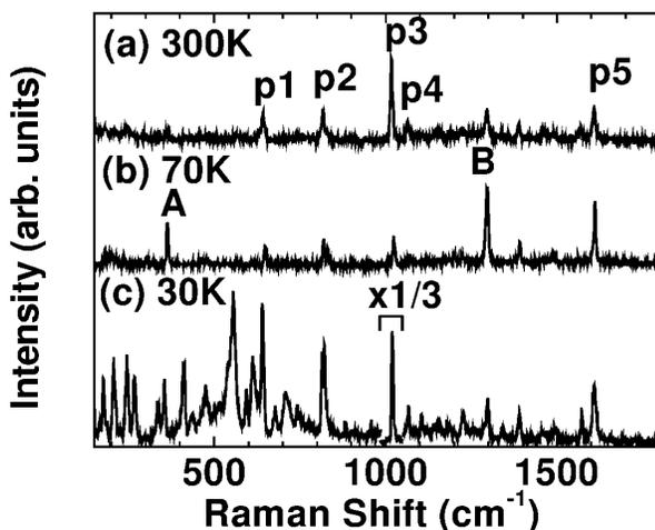
FIG. 2. Raman spectra of the  $[\text{Fe}(\text{2-pic})_3]\text{Cl}_2\text{EtOH}$  single crystal measured at (a) 300 K, (b) 70 K, and (c) 30 K. The light source is the second harmonic of cw- $\text{Nd}:\text{YVO}_4$  laser, 2.33 eV. The labels  $p1-p5$  show vibrations of the 2-picolylamine molecules. Labels  $A$  and  $B$  are described in the text.
