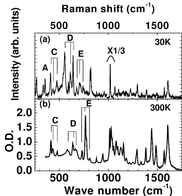
FIG. 3. (a) Raman spectrum measured in the photoinduced phase. (b) Infrared absorption spectrum of the  $[\text{Fe}(\text{2-pic})_3]\text{Cl}_2\text{EtOH}$  powder measured at 300 K. Labels  $C-E$  are described in the text.
