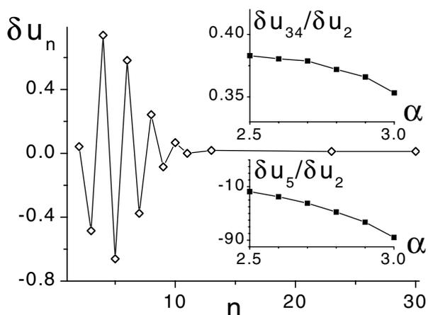
FIG. 3.  $y_n \equiv u_n/u_2$  as a function of the level number  $n$  and of the relative width of the barrier,  $\alpha$  (insets). Upper inset:  $y_{34}(\alpha)$ . The variation in the interval  $2.5 < \alpha < 3.0$  is less than 10%. Lower inset: linear dependence of  $\ln(y_5)$  on  $\alpha$ . Note that  $y_5(3)/y_5(2.5) \approx 5$ .
