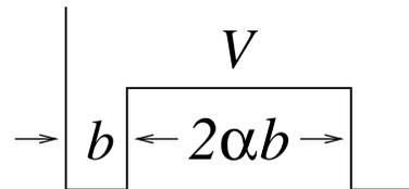
FIG. 2. Symmetric double-well potential with the well width  $b$ ; the barrier has a height  $V$  and a width  $2ab$ .
