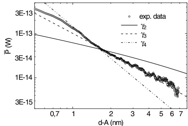
FIG. 3. Dissipation into the tip-sample interaction. Experimental data (circles) and calculated model curves (using the same parameters). The model assumes a damping coefficient which obeys an inverse power law with exponents  $n = 2$  (solid line),  $n = 3$  (dashed line), and  $n = 4$  (dash-dotted line). Parameters:  $f = 267\,220$  Hz;  $A = (24 \pm 2)$  nm;  $k_t = 40$  N/m;  $R = (35 \pm 5)$  nm;  $Q = 19\,050$ ; CPD compensated.
