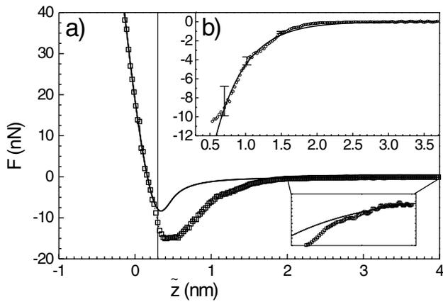
FIG. 2. (a) Reconstructed force curve from Fig. 1b together with a curve from the MYD model. (b) The difference between the two curves from (a). Parameters: Young's moduli: 42.7 GPa (Al), 62.5 GPa (Au); Poisson ratios: 0.46 (Al); 0.3625 (Au); Hamaker constant:  $3.5 \times 10^{-19}$  J.
