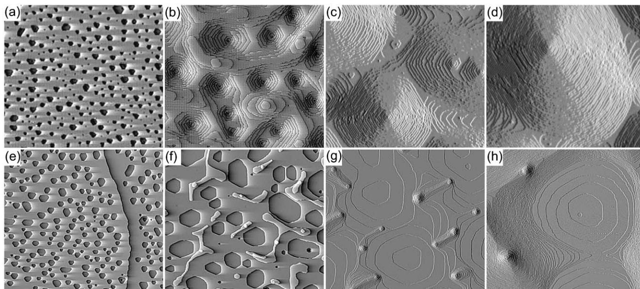
FIG. 1. STM topographs after erosion of (a) 0.26 ML, (b) 6.2 ML, (c) 66 ML, and (d) 333 ML at 600 K and of (e) 0.24 ML, (f) 6.3 ML, (g) 65 ML, and (h) 601 ML at 750 K. Topograph width 810 Å for (a)–(d) and 3460 Å for (e)–(h).
