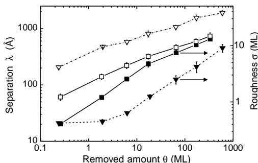
FIG. 2. Feature separation  $\lambda$  (left y-axis) and roughness  $\sigma$  (right y-axis) in dependence of removed amount  $\Theta$  at 600 K (down triangles and dashed lines) and 750 K (squares and full lines). Full symbols for  $\sigma$  and open symbols for  $\lambda$ . Lines to guide the eye.
