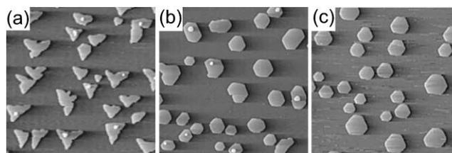
FIG. 3. (a) STM topograph after deposition of 0.2 ML Pt at 400 K. (b) Morphology created as in (a), but after subsequent annealing to 630 K for 180 s. (c) Morphology created as in (a), but after annealing to 700 K for 180 s. Topograph width 2200 Å.
