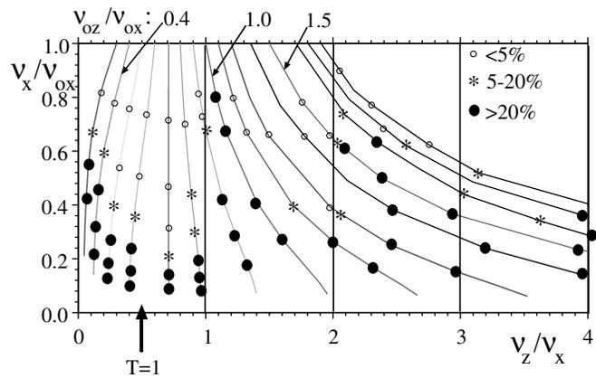
FIG. 3. Simulation results for initial  $\epsilon_z/\epsilon_x = 2$  (waterbag); markers indicate level of emittance growth in the initially colder direction (lines connecting markers indicate same focusing system  $\nu_{0z}/\nu_{0x}$  defined by the zero current value at  $\nu_x/\nu_{0x} = 1$ ).
