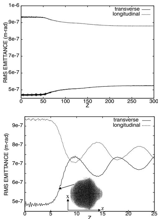
FIG. 2. rms emittances (upper trace in  $z$ , lower in  $x$ ) for  $\epsilon_z/\epsilon_x = 2$  (waterbag),  $\nu_{0z}/\nu_{0x} = 1.5$ , inside the resonance band of third order. Top:  $\nu_z/\nu_x = 2.04$  ( $T = 4.1 \rightarrow 2.6$ ); bottom:  $\nu_z/\nu_x = 2.94$  ( $T = 5.9 \rightarrow 1.6$ ). Units in  $z$  are transverse single particle periods without space charge ( $z - x$  scatter plot at period 6).
