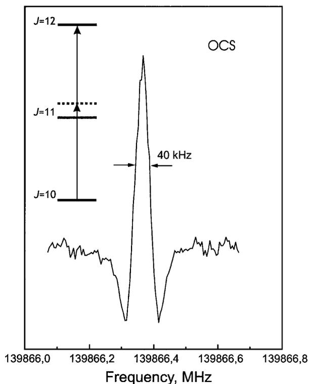
FIG. 3. The Doppler-free two-photon  $J = 12 \leftarrow 10$  transition of OCS. The linewidth is reduced by an order of magnitude in comparison with the Doppler width.
