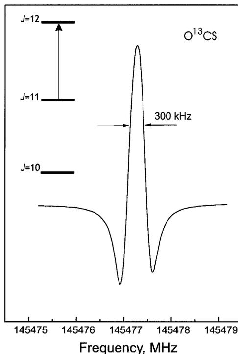
FIG. 2. The  $J = 12 \leftarrow 11$  transition of  $\text{O}^{13}\text{CS}$  measured in natural abundance of 1% with the intracavity jet millimeter wave spectrometer. The width of the absorption line is determined by Doppler broadening in the free jet.
