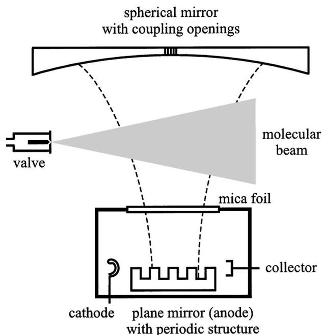
FIG. 1. Schematic representation of the intracavity jet arrangement of the OROTRON spectrometer. The geometry of the electromagnetic field in the resonator is shown by dashed lines. The periodic structure with the period of  $120\ \mu\text{m}$  is shown schematically on the surface of the plane mirror.
