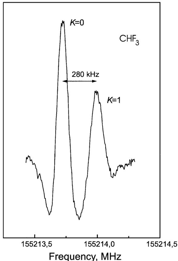
FIG. 4. The resolved  $K = 0$  and  $K = 1$  components of the Doppler-free two-photon transition  $J = 8 \leftarrow 6$  of  $\text{CHF}_3$ . The width of the two components is mainly determined by the collisional homogeneous broadening in the jet.
