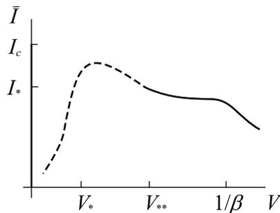
FIG. 1.  $I$ - $V$  characteristic given by the perturbation theory with  $\gamma \approx 2$  (solid line). The dashed line is a conjecture.
