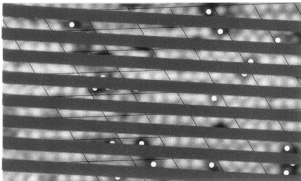
FIG. 3. Empty state STM image of Fig. 1(a) with a half transparent mask with a wavelength \lambda = 2\pi/\mathbf{K}_c . The dark segments of the mask cover 3/4 of all of the Si substitutional defects.
