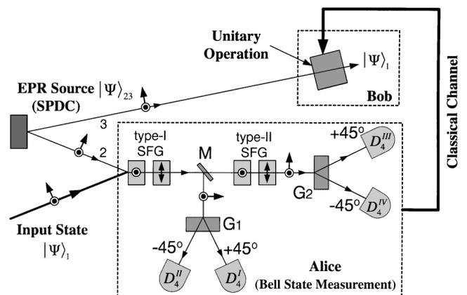
FIG. 1. Principle schematic of quantum teleportation with a complete BSM. Nonlinear interactions (SFG) are used to perform the BSM.  $\odot$  and  $\Downarrow$  represent the respective horizontal and vertical orientations of the optic axes of the crystals.
