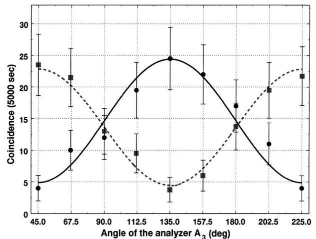
FIG. 2. The solid line (circled data points) is the joint detection rate  $D_4^I$ - $D_3$  for  $45^\circ$  linear polarization as an input state. The dashed line (square data points) is for  $D_4^{II}$ - $D_3$  for the same input state. The expected  $\pi$  phase shift is clearly demonstrated.
