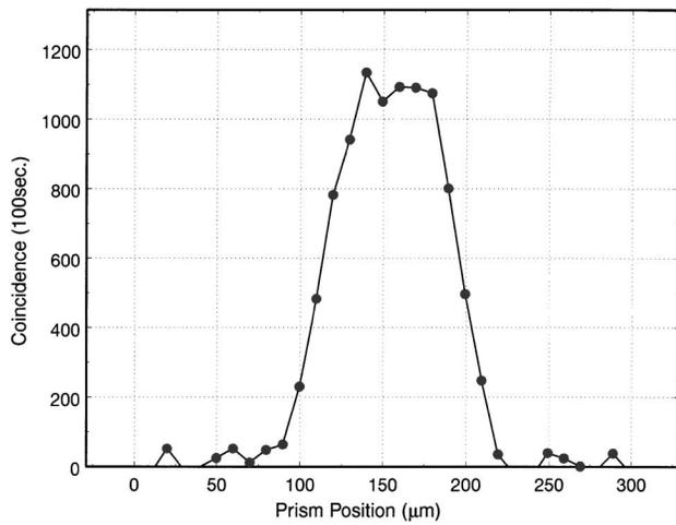
FIG. 5. SFG measurement as a function of the prism position. SFG is observed only when the input pulse and the SPDC photons overlap exactly inside the crystals.
