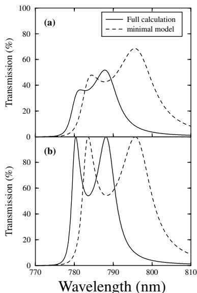
FIG. 3. Comparison between the calculated  $T_{00}$  within the full (solid line) and minimal (dashed line) models, for the system considered in Fig. 2, with  $d = 280$  nm. In panel (a) the dielectric constant is that of Ag, whereas in (b) absorption of Ag is neglected.
