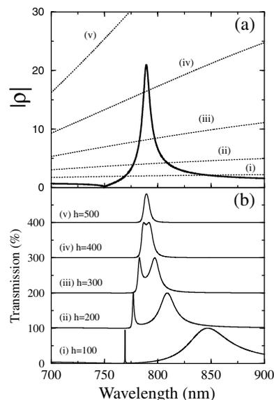
FIG. 4. (a)  $|\rho|$  versus  $\lambda$  for the parameters defined in Fig. 2, within the minimal model with no absorption (solid line). Also  $e^{|q_{z1}|h}$  for different values of  $h$  (in nm). (b)  $T_{00}$  versus  $\lambda$  for the metal thicknesses considered in panel (a) (successive curves being shifted by 100%).
