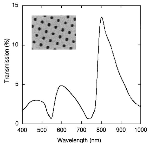
FIG. 1. Experimental zero-order power transmittance,  $T_{00}$ , at normal incidence for a square array of holes (lattice constant  $L = 750$  nm, average hole diameter of 280 nm) in a freestanding Ag film (thickness  $h = 320$  nm). Inset: electron micrograph of the perforated metal film.
