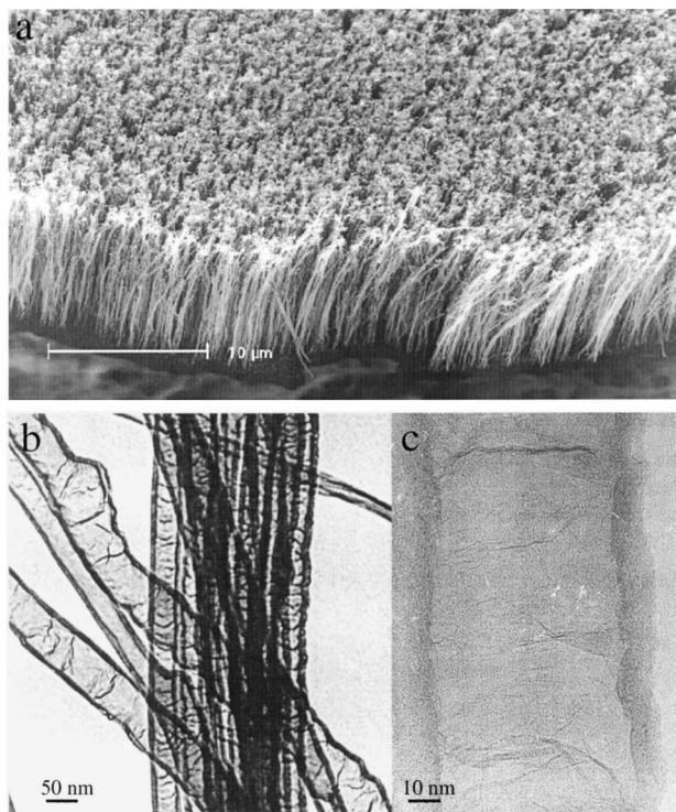
FIG. 1. (a) SEM image of the as-grown aligned carbon nanotube arrays on a quartz substrate. (b) Low-magnification TEM image showing the bamboolike structure of the carbon nanotubes. (c) A high-magnification TEM image showing the graphitic layered structures in the wall of a nanotube.
