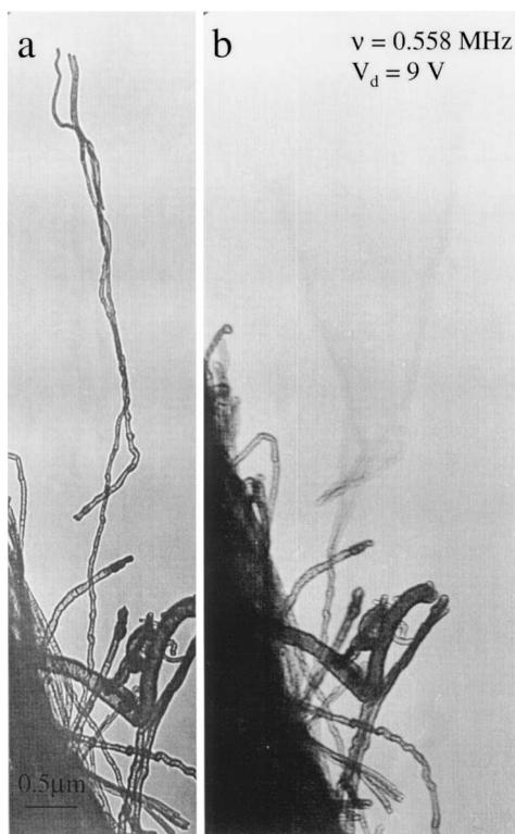
FIG. 4. (a) The stationary and (b) the first resonance mode of a carbon nanotube with another nanotube around its body. This is the principle of femtogram nanobalance of chain-structured large molecules.
