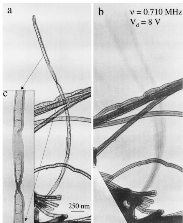
FIG. 3. A carbon nanotube at (a) the stationary and (b) the first resonance mode; (c) shows the presence of a necklike volume defect along the body of the nanotube.
