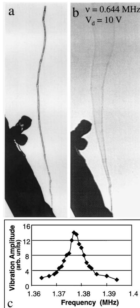
FIG. 2. A carbon nanotube at (a) the stationary and (b) the first resonance mode. (c) The FWHM of the resonance peak measured from another nanotube. The resonance occurs at 1.378 MHz.
