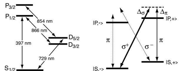
FIG. 1. Levels and transitions in  $^{40}\text{Ca}^+$  used in the experiment (left). Zeeman sublevels of the  $S_{1/2}$  and  $P_{1/2}$  states and lasers relevant for the cooling (right). The  $\sigma^-$  light arises from the  $\pi$  laser beam not being orthogonal to the quantization axis. For EIT cooling,  $\Delta_\pi = \Delta_\sigma$ .
