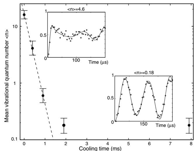
FIG. 4. Mean vibrational quantum number  $\bar{n}_y$  vs EIT cooling pulse length  $\tau$ . The insets show Rabi oscillations excited on the upper motional sideband of the  $|S, +\rangle \rightarrow D_{5/2}(m = +5/2)$  transition, after 0.4 ms (left) and 7.9 ms (right) of EIT cooling. A thermal distribution is fitted to the data to determine  $\bar{n}_y$ .
