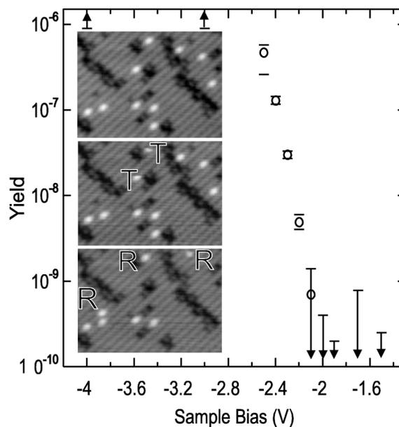
FIG. 1. Desorption yield for benzene/Si(100) as a function of sample bias at 22 K. Inset shows successive STM images (42 pA,  $-2.3$  V,  $150 \text{ \AA} \times 110 \text{ \AA}$ ,  $300 \text{ nm/s}$ ). Examples of molecules desorbing during the scan are marked “T” while readsorbed molecules are labeled “R”.
