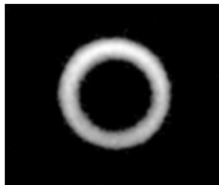
FIG. 1. 10 mm radius ringlike light output from a scintillator situated perpendicular to the axis 0.3 m behind the plasma lens.
