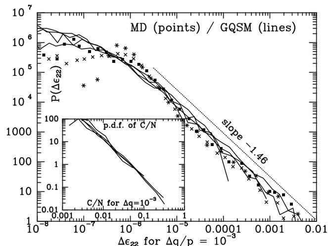
FIG. 5. Probability distribution function for strain increments  $\Delta \epsilon_{22}$  corresponding to  $\Delta q = 10^{-3}p$  obtained for the four values of  $N$  by GQSM (continuous curves) and for  $N = 1024$  (crosses) and  $N = 3025$  (square dots) by MD. The inset shows the distribution of  $C/N$ , where  $C$  is the number of lost contacts in one increment  $\Delta q$ , for the different system sizes.
