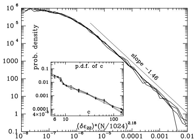
FIG. 4. Probability distribution function for rescaled strain increments  $\delta \epsilon_{22}(N/1024)^{2.18}$  for the four values of  $N$ . The inset displays the probability distribution function of the number  $c$  of lost contacts in one strain step for each system size.
