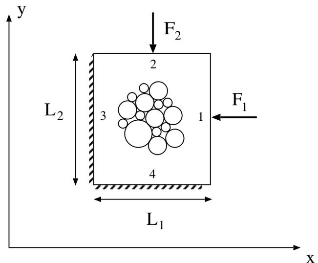
FIG. 1. Sketch of a biaxial compression test.
