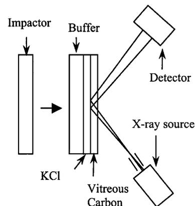
FIG. 1. Experimental arrangement used for x-ray diffraction measurements in shocked KCl.
