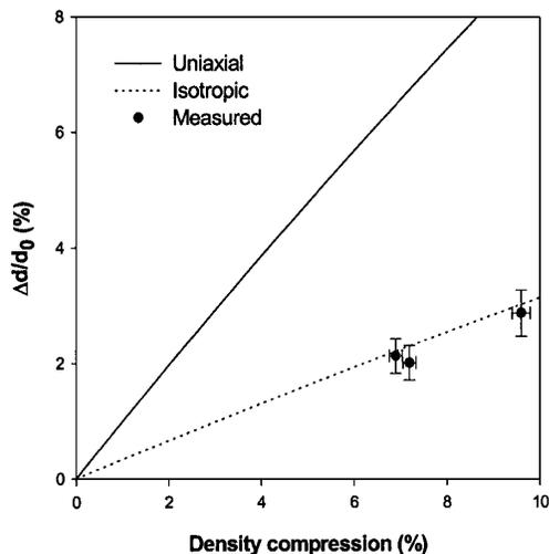
FIG. 4. Change in interplanar spacing versus density compression  $(V_0/V - 1)$  in phase I. Predictions based on uniaxial and isotropic compression of the unit cell are shown.
