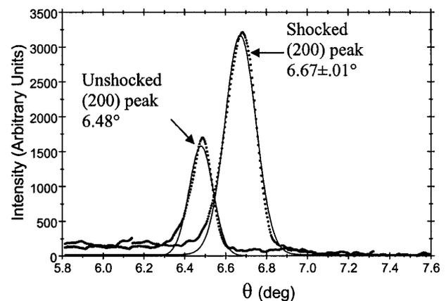
FIG. 3. Diffraction data from a typical experiment on KCl [100] in phase I (2 GPa at the KCl/VC interface). Intensity of the shocked peak was higher because the x-ray tube was positioned closer to the angle expected for the shocked state.
