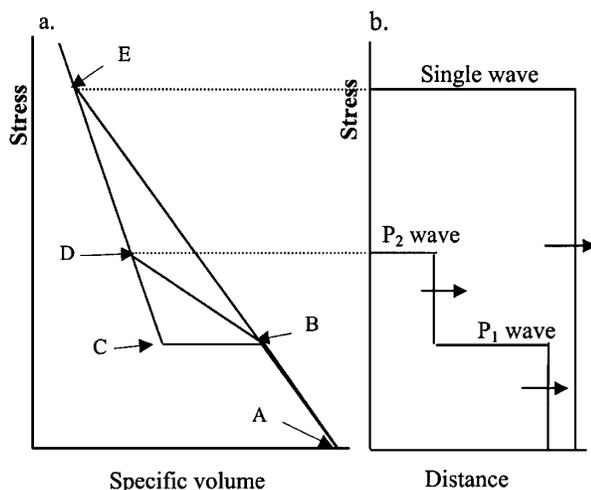
FIG. 2. Schematic representation of (a) compression curve for KCl and (b) stress-distance profiles.
