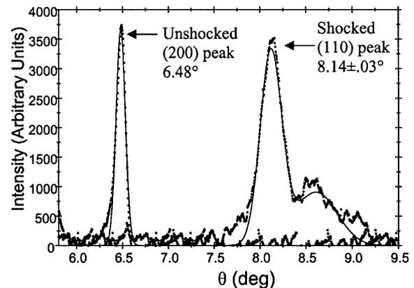
FIG. 5. Diffraction data showing the phase transition in KCl shock compressed along [100] to 6.9 GPa. Solid curves are Gaussian fits to the data.
