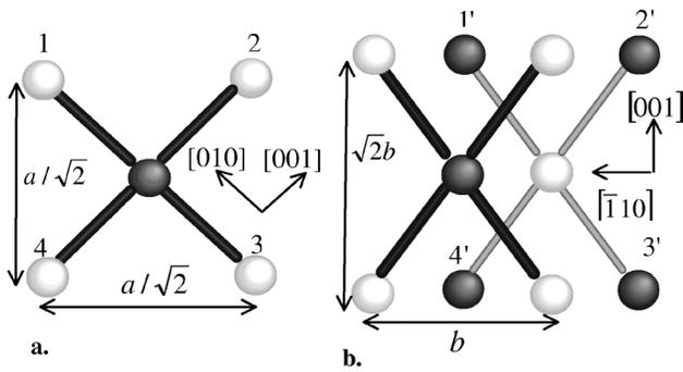
FIG. 6. Atomic arrangements as viewed along the direction of shock propagation. Potassium atoms are shown in light color and chlorine atoms are shown in dark color. (a) Front (100) plane of the NaCl structure along with the [100] axes. (b) First and second (110) planes of the CsCl structure. Atoms in the first plane are linked by darker colored bonds.
