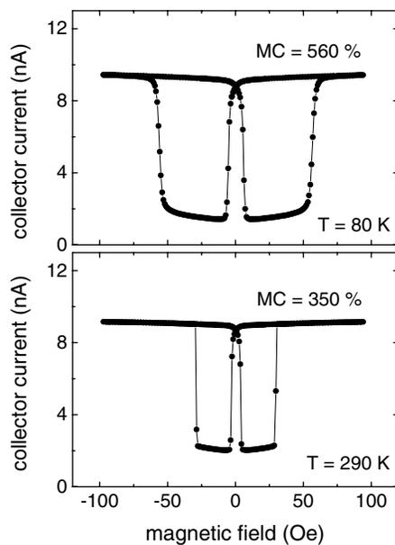
FIG. 1. Collector current versus magnetic field at  $T = 80$  K (top) and  $T = 290$  K (bottom), for a spin-valve transistor with a soft NiFe/Au/Co spin-valve base.  $I_E = 2$  mA;  $V_{BC} = 0$ .
