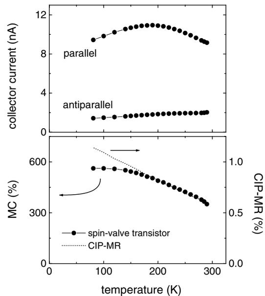
FIG. 2. Temperature variation of collector current  $I_C$  for parallel and antiparallel alignment (top panel) and the magnetocurrent (bottom panel, symbols).  $I_E = 2$  mA and  $V_{BC} = 0$ . Also shown is the much smaller CIP-MR of an identical spin valve (dashed line in bottom panel and right vertical scale).
