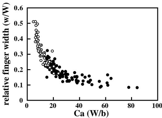
FIG. 5. Relative finger width as a function of  $Ca(W/b)$  for channel widths of  $W = 4$  (●) and  $2$  cm (○) and plate spacings of  $b = 0.125, 0.25, 0.5, 0.75,$  and  $1$  mm.
