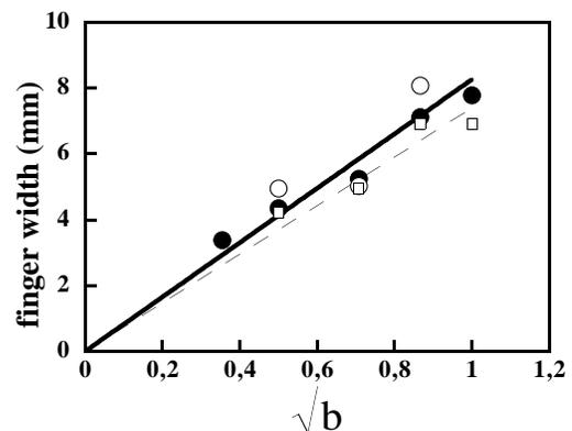
FIG. 4. Finger width versus  $\sqrt{b}$  for channel widths of 4 cm ( $\bullet$ ) and 2 cm ( $\circ$ ) for the gel and for the emulsion ( $\square$ ) for  $W = 4$  cm.
