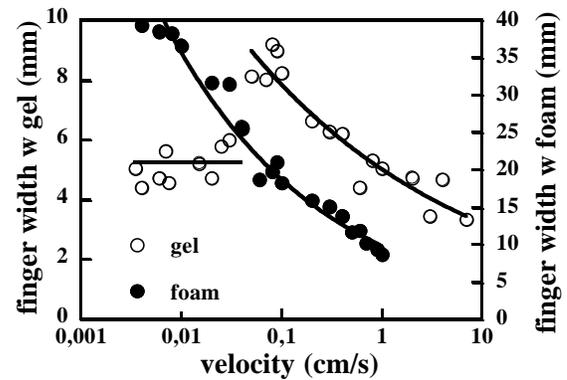
FIG. 2. Finger width versus finger velocity (on a logarithmic scale) for the gel (open circles) and for the foam (filled circles) for  $W = 4$  cm and  $b = 0.5$  mm.
