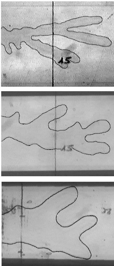
FIG. 1. Snapshots of the viscous fingers for gel at low velocities ( $U < 0.01$  cm/s) for  $W = 4$  cm; plate spacings of  $b = 0.125, 0.25,$  and  $0.75$  mm from top to bottom.
