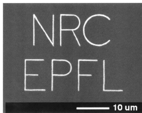
FIG. 3. SEM micrograph of selectively electrodeposited Cu letters on p -type Si(100). The latent letter patterns were FIB written with Si ++ ions at 200 keV and a dose of 3 \times 10^{14} cm -2 . Then the maximum damage zone was exposed using a uniform chemical Si etch and Cu was deposited by polarizing the sample in 0.1M H 2 SO 4 + 0.01M CuSO 4 from -0.5 to -2 V SCE. The letters were implanted with a nominal ion beam width of 200 nm; the width of the deposited Cu letters results as 200–300 nm.
