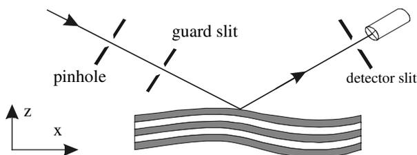
FIG. 1. Scheme of the experimental setup.
