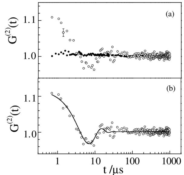
FIG. 2. Autocorrelation function for a 95 layer film (thickness  $0.27 \mu\text{m}$ ) in the Sm-A phase at  $50.1^\circ\text{C}$ . (a) Raw data (open dots) and reference signal from the NiC multilayer (filled dots). (b) Normalized correlation function obtained by dividing the raw data by the NiC reference signal; solid line is a fit to Eq. (1). For error bars, see text.
