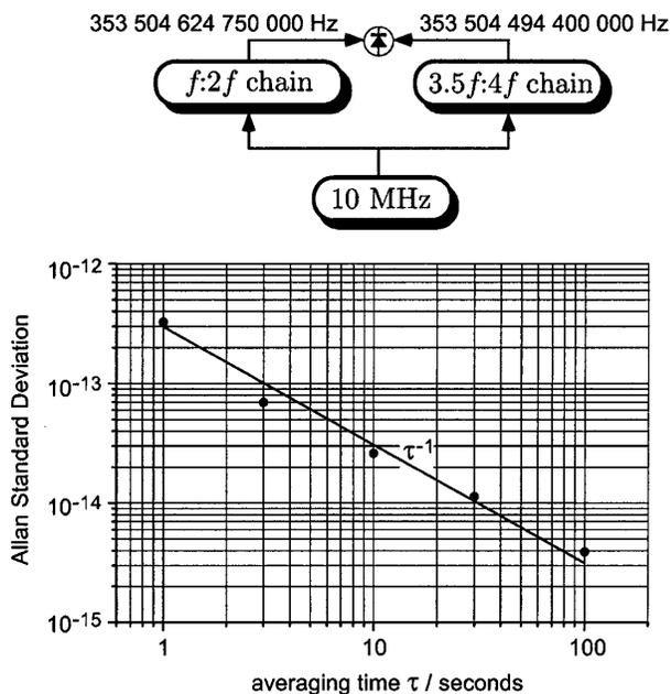
FIG. 3. Top: The setup is shown schematically with the  $f:2f$  and the  $3.5f:4f$  chains as detailed in Figs. 1 and 2, respectively. The graph below shows the measured relative Allan standard deviation derived from the comparison of the two frequency chains. The values are also stated in Table I.
