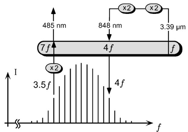
FIG. 2. The first realization of the novel frequency chain that has been used in Refs. [5,22] uses an optical frequency interval divider (oval symbol) [24] that fixes the relation between the frequencies  $f$ ,  $4f$ , and  $7f$ . The 3.39  $\mu$ m laser at  $f$  is locked through the divider after the frequency comb locked  $3.5f$  on  $4f$ .
