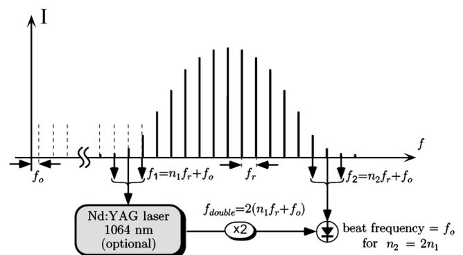
FIG. 1. The  $f:2f$  interval frequency chain is based on the stabilization of the interval between an optical frequency  $f$  and its second harmonic  $2f$  with the help of a fs frequency comb. Once the offset frequency and repetition rate are locked, all the modes in the comb can be used for optical frequency measurements.
