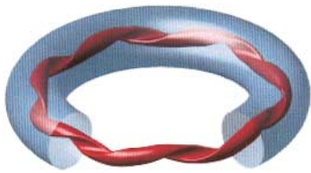
FIG. 3 (color). Schematic view of a n = 7 helical structure inside the RFX vessel.
