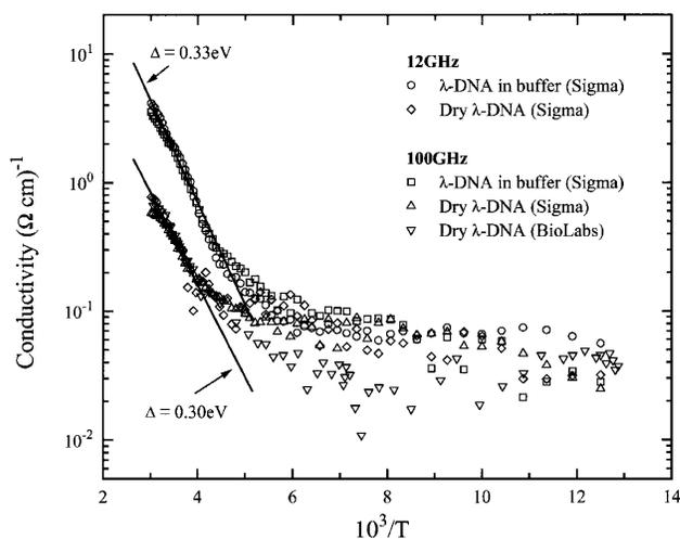
FIG. 2. Conductivity of dry  $\lambda$ -DNA and  $\lambda$ -DNA in buffer versus inverse temperature as measured at 12 and at 100 GHz. The magnitude of the conductivity was determined at 12 GHz, and the 100 GHz data were normalized to the 12 GHz results at room temperature. The full lines are Eq. (2) with  $\Delta$  values as given in the figure and  $\sigma_0$  values as given in the text.
