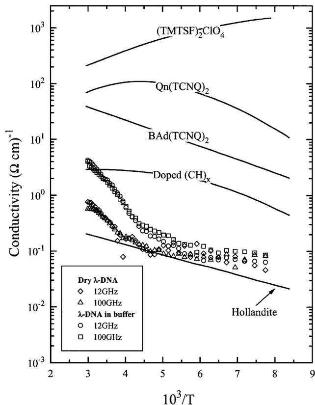
FIG. 3. Conductivity of  $\lambda$ -DNA versus the inverse temperature as measured at 12 and 100 GHz, together with the electrical conductivity of several organic linear chain compounds and an inorganic superionic conductor.
