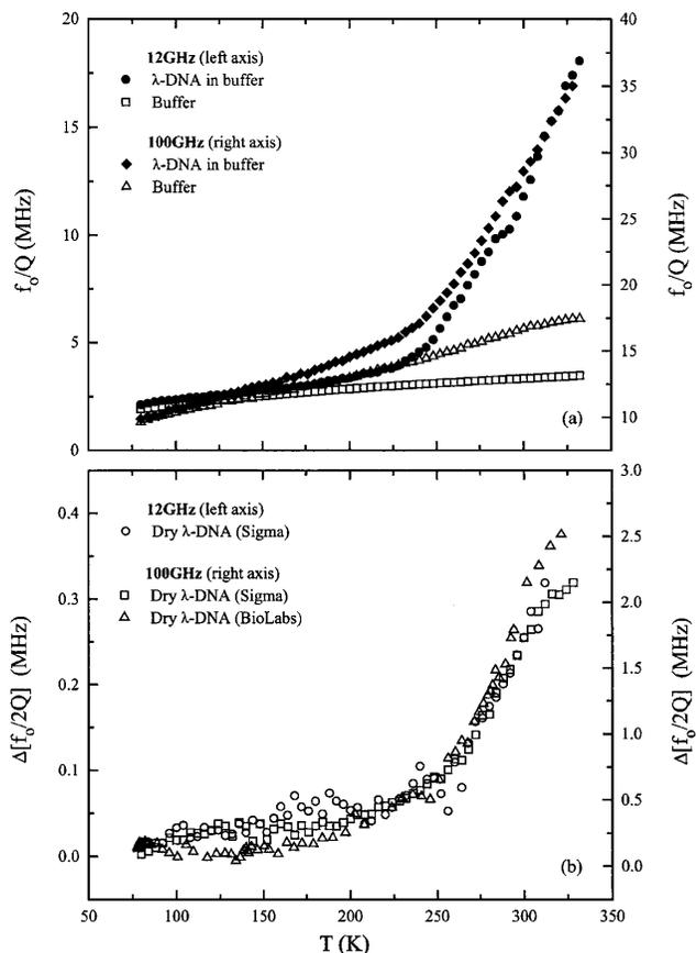
FIG. 1. (a) Temperature dependence of the excess cavity loss for the cavity loaded with the buffer material and the cavity loaded with lyophilized  $\lambda$ -DNA in buffer [13] measured at 12 and at 100 GHz. Buffer materials prepared in slightly different ways all display temperature independent loss, but of somewhat varying magnitude. (b) Temperature dependence of the excess cavity loss for a cavity loaded with dry  $\lambda$ -DNA [14] measured at 12 and at 100 GHz.
