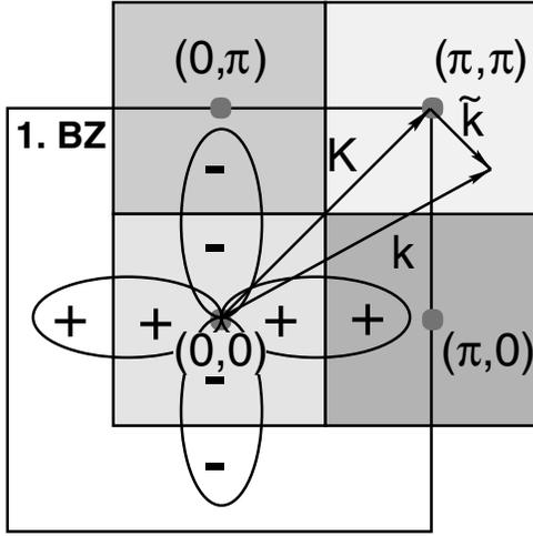
FIG. 1. Choice of the  $N_c = 4$  cluster  $\mathbf{K}$  points (filled circles), corresponding coarse graining cells (shown by different fill patterns), and a sketch of the  $d$ -wave symmetry of the order parameter.
