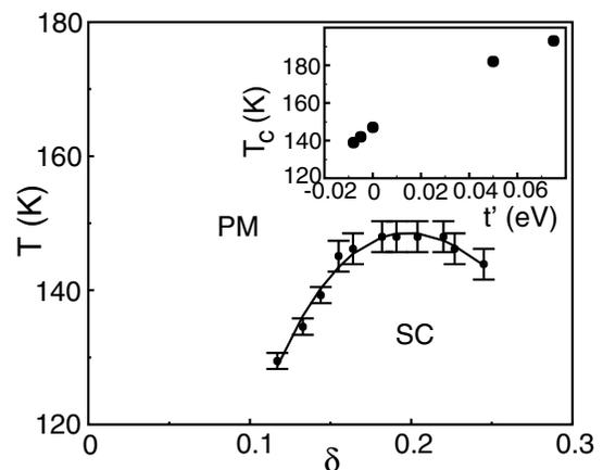
FIG. 4. Temperature-doping phase diagram for the 2D Hubbard model via DCA for a  $N_c = 4$  cluster. The nearest neighbor hopping  $t = 0.25$  eV, next nearest neighbor hopping  $t' = 0$ , and the Coulomb repulsion  $U = 3$  eV. The error bars result from the finite resolution in temperature. Inset: Transition temperature  $T_c(t')$  for fixed doping  $\delta = 0.18$  as a function of the next nearest neighbor hopping amplitude  $t'$ .
