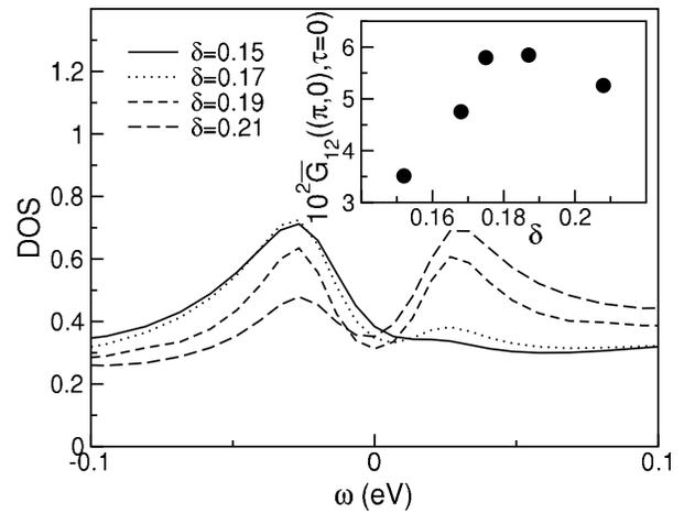
FIG. 3. Density of states in a narrow region at the Fermi energy for the same parameters as in Fig. 2 but for various dopings. The gap size and the density of states at  $\omega = 0$  are independent of doping. Inset: Equal time coarse grained anomalous Green function  $\bar{G}_{12}(\mathbf{K}, \tau = 0)$  at  $\mathbf{K} = (\pi,0)$ .
