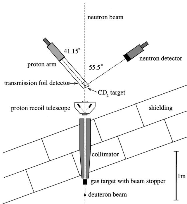
FIG. 1. Schematic drawing of the experimental setup, approximately to scale.
