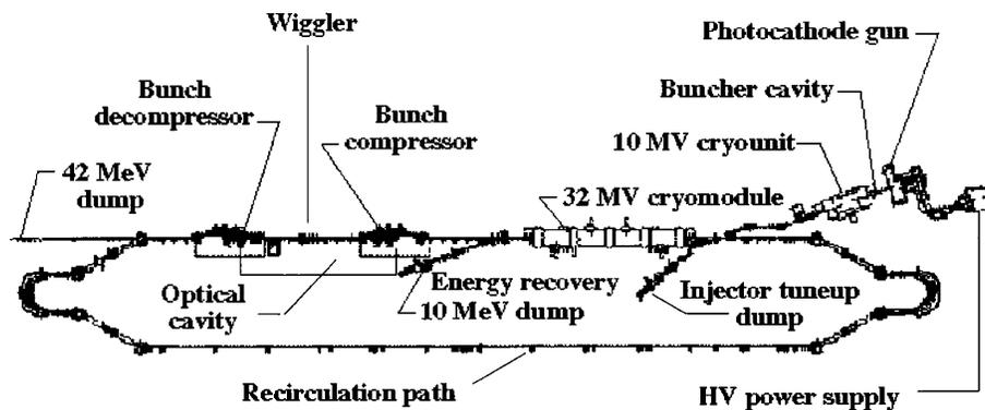
FIG. 1. Schematic of IR Demo; dimensions of the recirculation loop are roughly  $49 \text{ m} \times 6 \text{ m}$ .
