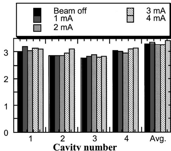
FIG. 2. Cryomodule rf power in watts versus recirculated current while lasing. The first four of eight cavities and the average of all eight cavities are shown. Variations in power are comparable to fluctuations due to microphonics.
