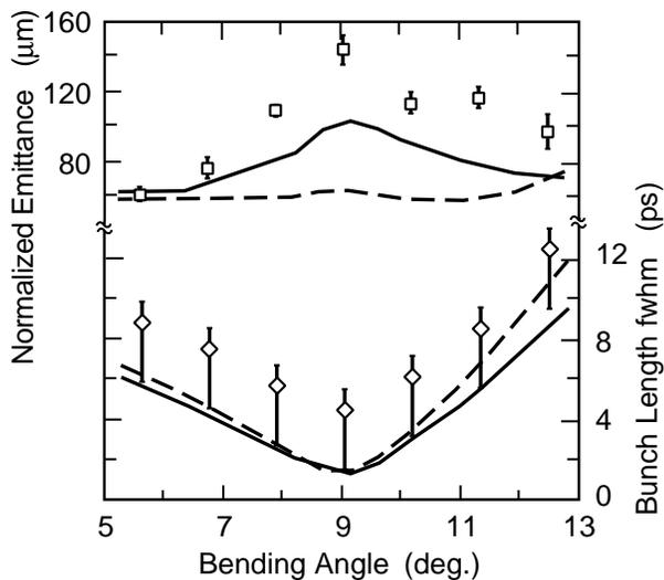
FIG. 4. Comparison of the measured rms horizontal emittance (squares) and rms bunch length (diamonds) with PARMELA (dashed lines) and CSR-TRACK (solid lines) for 6 nC per bunch.
