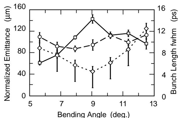
FIG. 1. Measured rms normalized horizontal (squares) and vertical (circles) emittances, and rms bunch length (diamonds) versus angle in the first bend of the compressor with 6 nC.
