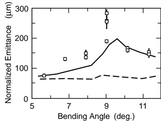
FIG. 5. Comparison of the measured rms horizontal emittance (squares) with PARMELA (dashed line) and CSR-TRACK (solid line) for 16 nC per bunch.
