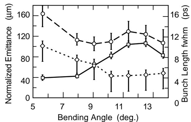
FIG. 3. Measured rms horizontal (squares) and vertical (circles) emittances, and rms bunch length (diamonds) versus current in the first bend of the compressor with 6 nC per bunch and a smaller energy correlation.
