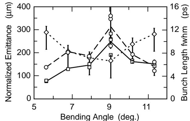
FIG. 2. Measured rms horizontal (squares) and vertical (circles) emittances, and rms bunch length (diamonds) versus angle in the first bend of the compressor with 16 nC.
