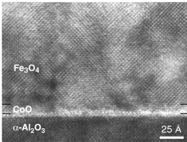
FIG. 5. High-resolution TEM image of a [111] oriented 140 Å  $\text{Fe}_3\text{O}_4$ /10 Å CoO bilayer grown on (0001)  $\alpha\text{-Al}_2\text{O}_3$ .
