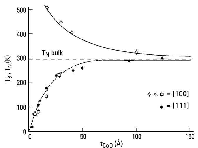
FIG. 4. Both the measured CoO ordering temperatures,  $T_N$  ( $\diamond$  symbols) and blocking temperatures ( $\bullet$ ,  $\circ$ , and  $\square$  symbols) are given versus the thickness of the CoO layer for the  $\text{Fe}_3\text{O}_4/\text{CoO}$  system. Note the divergence of the two curves, indicating that the measured reduction of  $T_B$  is not due to a reduction of the ordering temperature at low  $t_{\text{CoO}}$ .
