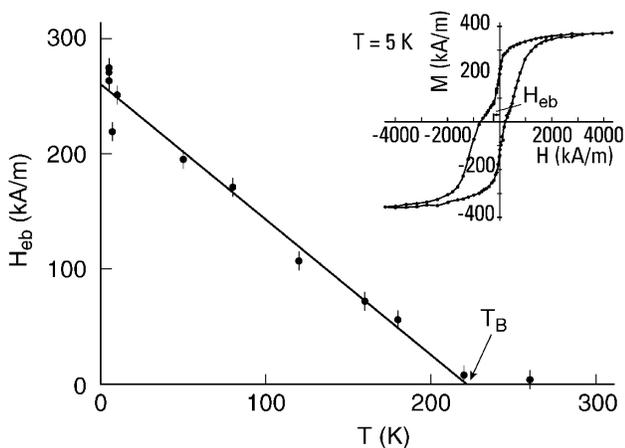
FIG. 1. The exchange biasing field  $H_{\text{eb}}$  versus temperature  $T$  for a [111] oriented  $125 \text{ \AA}$  Fe<sub>3</sub>O<sub>4</sub>/33  $\text{\AA}$  CoO bilayer. Note the linear dependence of  $H_{\text{eb}}$  on  $T$ . The biasing vanishes at the blocking temperature  $T_B = 220 \pm 10 \text{ K}$ . The inset shows the hysteresis loop at 5 K after cooling from 350 K in a field of 4400 kA/m.
