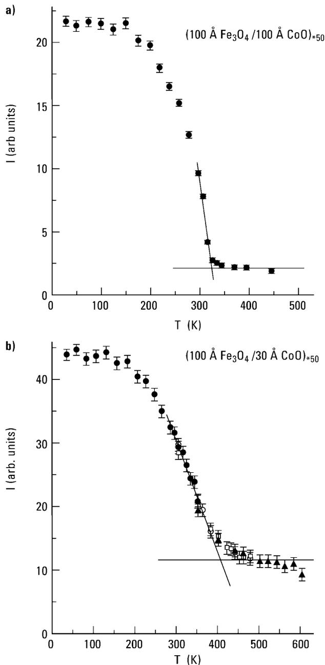
FIG. 3. The intensity  $I$  of the (111) reflection as a function of  $T$  for a  $(100 \text{ \AA} \text{ Fe}_3\text{O}_4/100 \text{ \AA} \text{ CoO})_{\times 50}$  (a) and a  $(100 \text{ \AA} \text{ Fe}_3\text{O}_4/30 \text{ \AA} \text{ CoO})_{\times 50}$  (b) multilayer. Note the drop in  $I$  around 410 K in the latter. (The various symbols denote the results from different experimental runs.)
