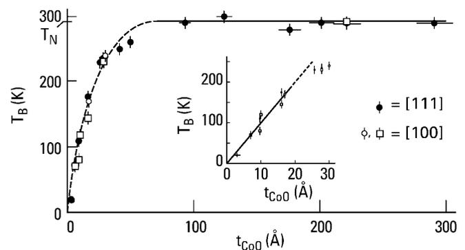
FIG. 2. Blocking temperature  $T_B$  as a function of the CoO layer thickness  $t_{\text{CoO}}$  in Fe<sub>3</sub>O<sub>4</sub>/CoO bilayers for two orientations. The curve is a guide to the eye. Note that there is no measurable influence of the substrate used: Al<sub>2</sub>O<sub>3</sub> ( $\bullet$ ), SrTiO<sub>3</sub> ( $\circ$ ), or MgO ( $\square$ ). The inset shows that the  $T_B$  data display a linear dependence on  $t_{\text{CoO}}$  for  $t_{\text{CoO}} < 20 \text{ \AA}$ .
