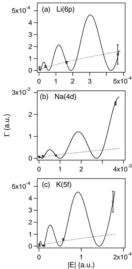
FIG. 3. Widths of doubly excited states versus the absolute values of their energies for a given series of states in (a)  $\text{Li}^-$ , (b)  $\text{Na}^-$ , and (c)  $\text{K}^-$ . Circles represent experimental data. Fits of experimental data to Eqs. (7) and (9) are shown by the solid and dotted curves, respectively.
