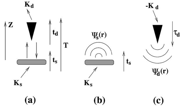
FIG. 2. (a) General SNOM setup with directional illumination and detection. (b) Illustration of the meaning of the sample wave function  $\Psi_s$ . (c) Illustration of the meaning of the tip wave function  $\Psi_d$ .
