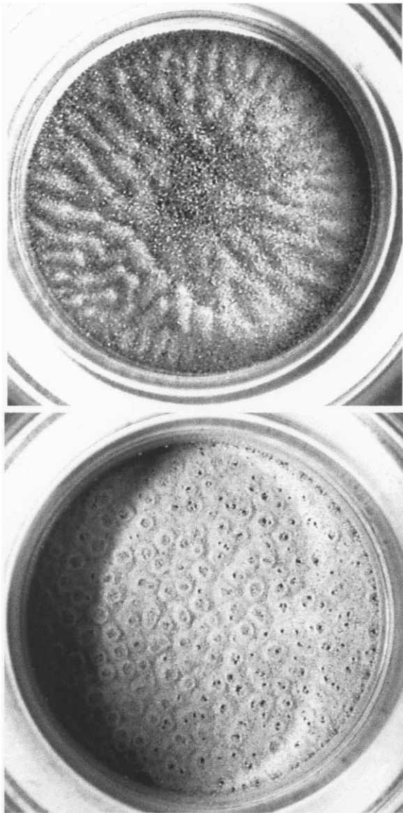
FIG. 4. The top photograph shows ripples obtained by using fast transient air pulses. The bottom photograph obtained with a continuous air flow exhibits small craters (black points) sitting at the center of the myriad of small fixed volcanoes.
