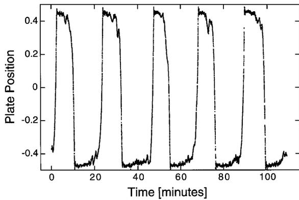
FIG. 3. Floater position, normalized by the cell length, versus time. The aspect ratio is 3.3, coverage ratio 0.36, and Rayleigh number  $2.0 \times 10^8$ .
