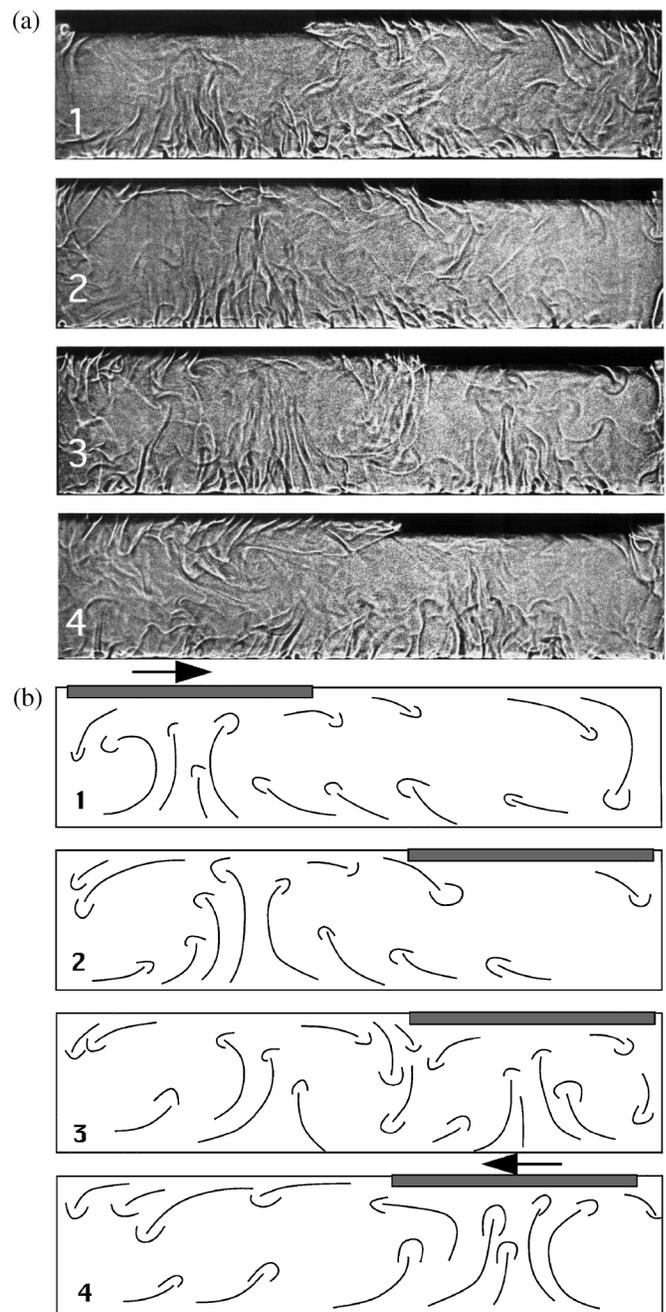
FIG. 2. (a) Four shadowgraphs at different times within half a period. (b) Sketches of the shadowgraphs illustrating the main flows. Aspect ratio is 4.0, coverage ratio 0.38, and Rayleigh number  $3.2 \times 10^8$ .
