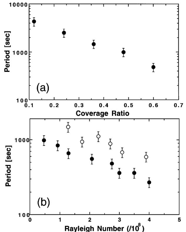
FIG. 4. (a) Period of oscillation of the floater as a function of the coverage ratio, where Rayleigh number is  $10^8$ . (b) Period as a function of the Rayleigh number. Open circles correspond to a floater of coverage ratio 0.36; close circles correspond to 0.48.
