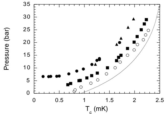
FIG. 1. The pressure is plotted versus  $T_c$  for different aerogel samples. The legend is as follows: filled squares are cell *A* (98% aerogel) [1], filled triangles are cell *B* (98% aerogel) [4], filled circles are for cell *C* (98% aerogel) [5], and empty circles are cell *D* (99.5% aerogel). The solid line is the superfluid transition curve for bulk  $^3\text{He}$ .
